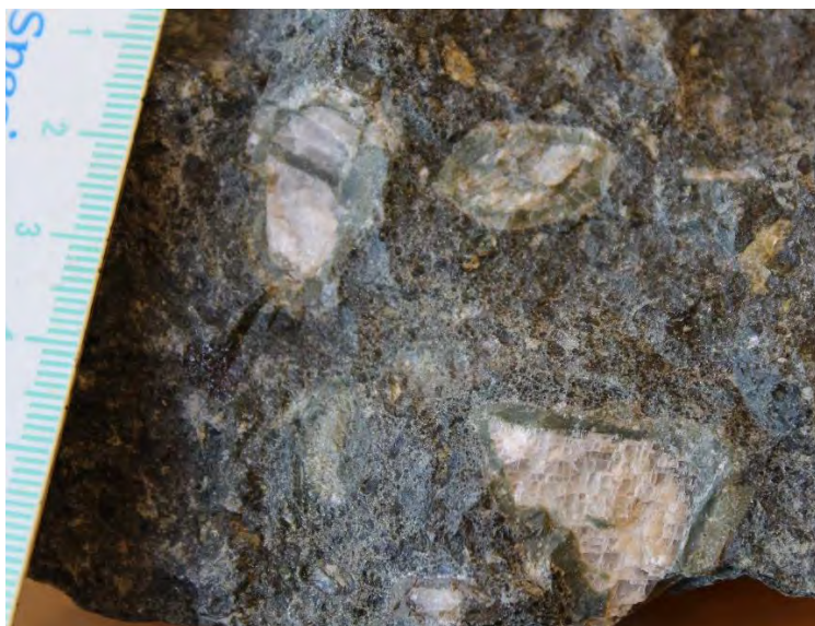
Figure 1. Photograph of carbonate nodules within a hypabyssal kimberlite block from the Bultfontein kimberlite. Note the distinct green reaction margins. Scale is in cm.
