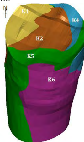
Figure 1. The different lithofacies of the Main Liqhobong Kimberlite Pipe. The pipe's surface diameter is ~300m.
