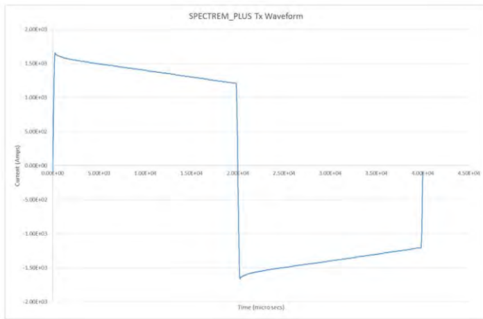
Figure 2: SPECTREM PLUS transmitter waveform
