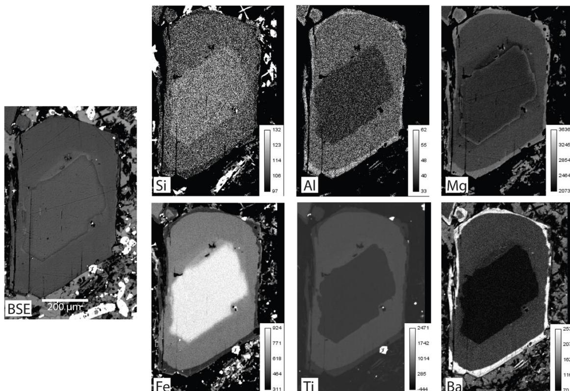
**Figure 1:** Back-scattered electron (BSE) image and EPMA elemental distribution maps of phlogopite in ultramafic lamprophyres (UML) in the Yilgarn Craton. The coloured scales on the right bottom of each panel indicate the relative concentration of each element
