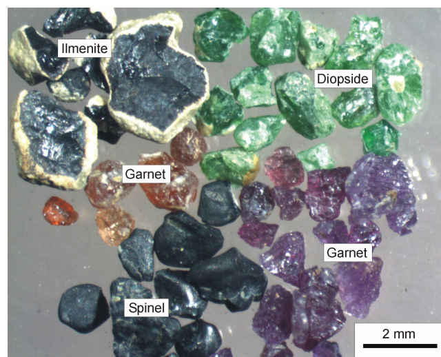
Fig.3. Photograph of indicator minerals from the heavy concentrate of a TKF kimberlite. Note the white coating on ilmenite macrocrysts.
