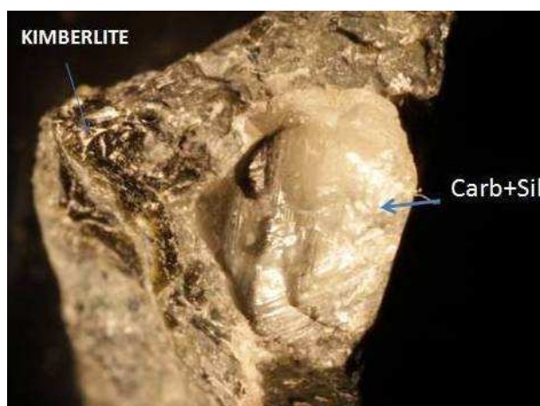
Figure 2. Thick carbonate-silicate shell of diamond (pipe "Mir")
