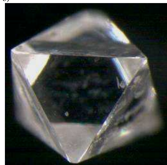
Fig. 5. Diamonds of first (a) and second (b) generation in eclogite xenolith, sample UG-31. Size of diamonds is 2.0 and 0.5 mm, respectively.
