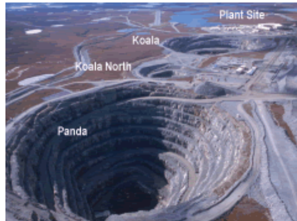
Figure 1. Oblique view looking south across the central development area at Ekati. The Panda open pit is in the foreground, the Koala North underground project is located beneath the existing test pit mid-frame, and the Koala pit and Ekati plant site are in the background. Photo taken in mid-2002.
