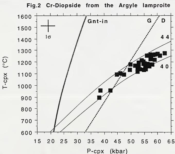
**Figure 2:** Pressure-temperature plot for xenocrystic Cr-diopside from the Argyle olivine lamproite pipe showing deep mantle sampling in the diamond stability field and a geotherm of ~42 mW/m<sup>2</sup>.
