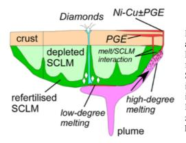
**Figure 2:** Interactions between magmas and the base and edges of cratonic roots. Plume magmatism triggers kimberlite formation and flows to areas of thinner SCLM where melting is focused. Variable interaction of melts with crust and SCLM influences Ni-Cu and PGE deposit genesis. Lithosphere-scale discontinuities and zones of weakness can focus the locus of kimberlite eruption.
