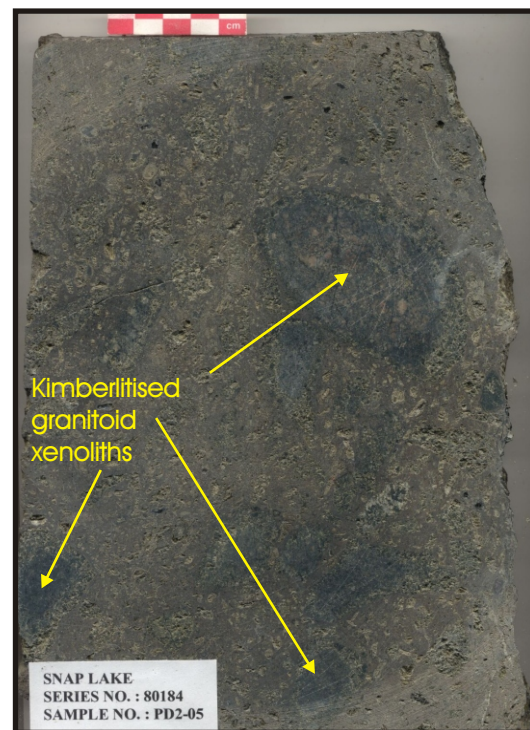
Figure 4: Hypabyssal granitoid-rich breccia from the lower tunnel. The sample contains numerous kimberlitised granitoid xenoliths in an altered brown matrix.
