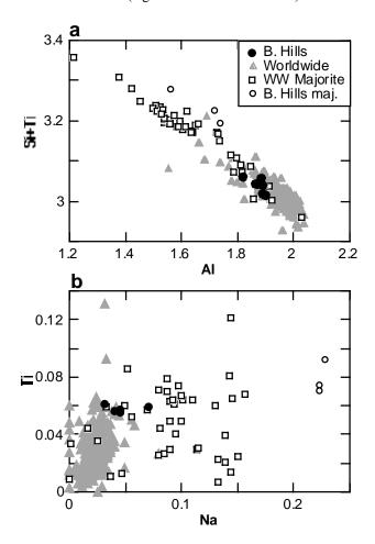
Figure 1. Compositions of eclogitic garnet and majorite in K10 and K14 diamonds compared to worldwide eclogitic garnet and majorite inclusions in diamond (in cations per formula unit).
